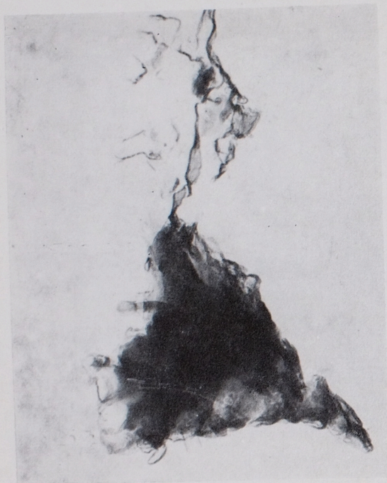
Phot. 3. Grains of iron oxides with sharp lines and visible triangular angles. \times 80\ 000
