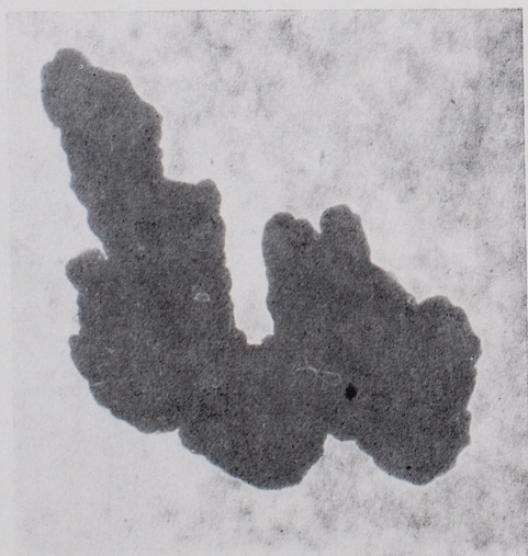
Phot. 5. Plates of iron oxides with irregular outlines. \times 80\ 000
