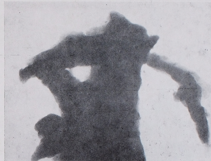
Phot. 1. Aggregate of grains of iron oxides with irregular shapes. \times 48\ 000
