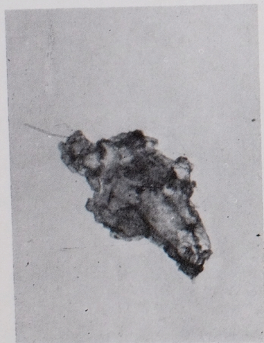
Phot. 4. Particles of incrustation formed from grains with flaky structure. \times 100\ 000
